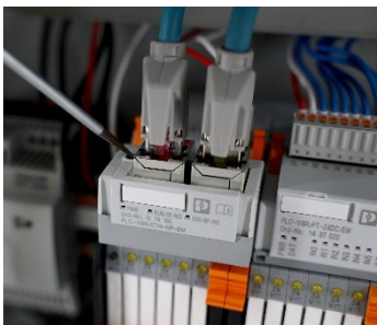
Multi-protocol connection to the network module
